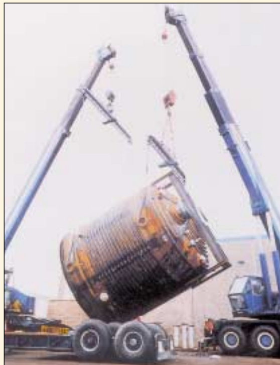
AstroCosmos fabricated this zirconium-clad reactor vessel, which has operated successfully for five years.
