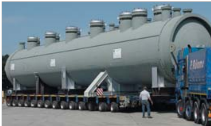
DMC Nobelclad produced the titanium-steel clad plates for this autoclave (4.3 m diameter x 29 m long). According to DMC's John Banker, the exceptionally uniform strength and ductility of Wah Chang's Grade 17 Titanium has helped to make the project one of "the most successful large titanium clad jobs ever".
