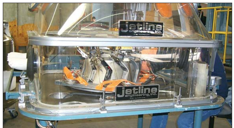
Figure 8. Chamber welding is ideal for small complex work
