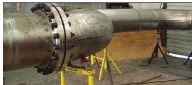
20 in. (0.5 m) diameter Zr 702 pipe spool
