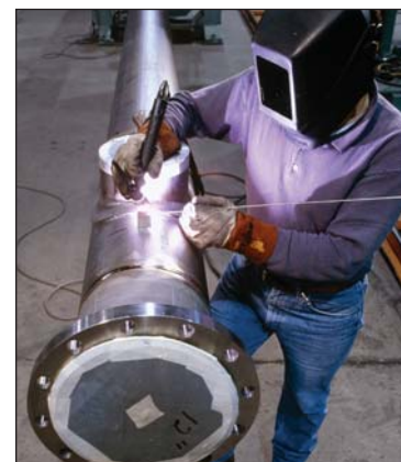
Open air manual GTA welding of zirconium pipe
