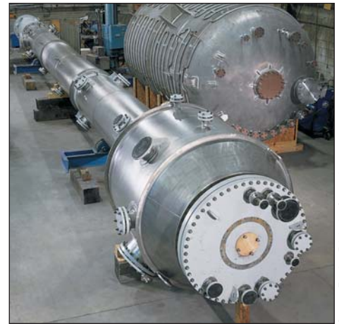
Zr 702 extraction column
