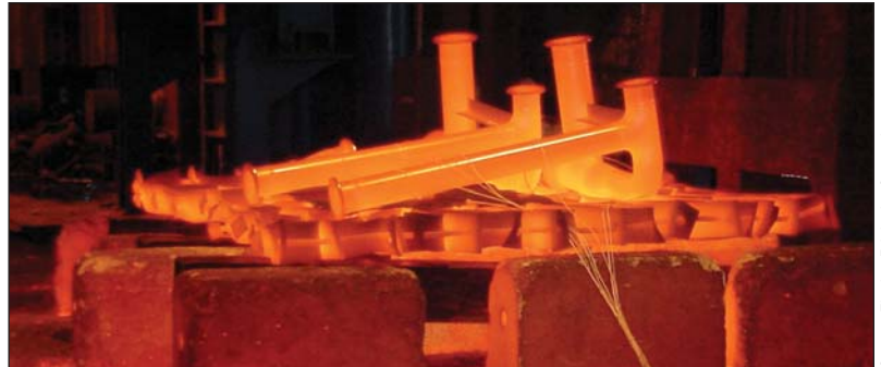
Stress relief heat treatment of Zr 705 prevents delayed cracking
